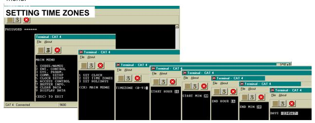
A time zone is a period of time that limits when the CAT is valid. Use this to control access to a facility, when a given condition is valid, based on:
