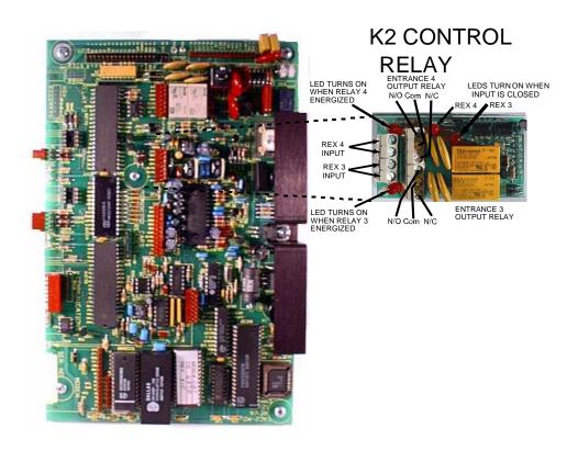
The relay capabilities are 24 volts LED TURNS ON AC or DC at 3 amps. Form "C" (N/ WHEN RELAY 4 O) AND (N/C) contacts are on the ENERGIZED control output relay for controlling devices.
