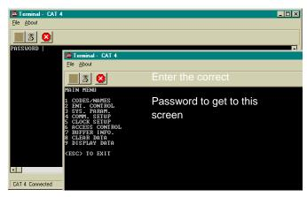
If you make a mistake at any time, before pressing the <Enter> key you can correct it by using the <Backspace> or <BkSpc> key. This will depend on what it is called on your keyboard.
