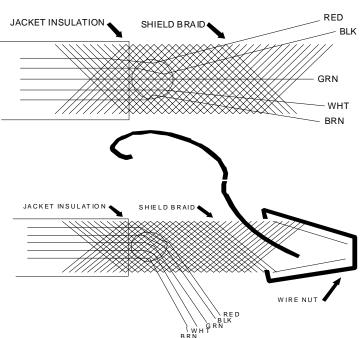
Poke a hole in the braid as shown at left. Spread the braid open, so the conductors are visible. Peel the conductors out, taking care not to damage the insulation on the conductors.
