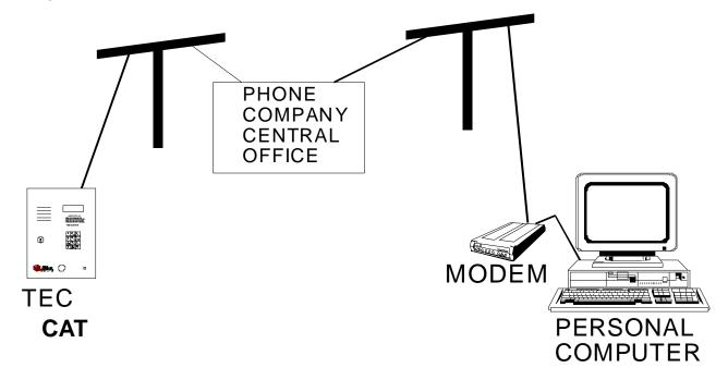
For computers equipped with Windows, the optional Selcom 2000 or Newer may be used to control the CAT series unit. This program has many features, including automatic upload (sending information to the CAT unit) and automatic download (getting information from the CAT series unit).
