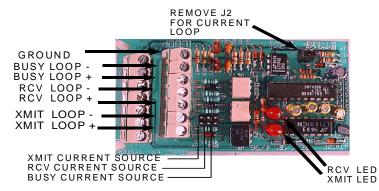
A recommended cable is Belden # 8770. The shield connects to the ground lug on the terminal barrier strip inside the CAT housing (see Pg.7).
