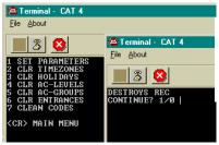
The Clear Data selections enable you to reset the unit to zero values or factory defaults if zero would not be acceptable. A warning message requiring you to press "1" is present for each action. Press "Enter" key to return to the Main menu.
