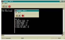
The Entry Control menu comes with factory defaults that should be sufficient for most installations. These default values are shown on Pg. 51 and 52. Some functions work with options that may not be present on your CAT unit. To get the menu at left, press "2" and then select the entrance to modify, The CAT unit can support up to 16 entrances with options installed.
