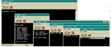
Access Levels are used to attach Time Zones to specific Entrances. Only one Time Zone is allowed per Access Level. Any combination of entrances may be selected, but at least one entrance must be selected, or the affected Access Level will not function. From one to sixteen entrances may be assigned to an Access Level. Different combinations of control may be created. Do this by assigning one entrance a Time Zone
