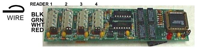
Strip 3/16" insulation from the conductors. Fold the stripped portion of the conductor over the insulated portion. Insert the wire in the clamps of the screw terminals on the card reader board and clamp down by screwing the terminal screw tightly. This ensures a good mechanical connection and an electrical connection that will keep the small wires from breaking.
