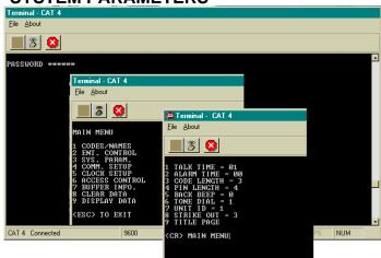
The System Parameters menu comes with factory defaults that should be sufficient for most installations. These default values are shown on Pg. 51 and 52. Some functions work with options that may not be present on your CAT. For example, selection 2 Alarm Time is not valid unless the optional alarm control relay (OPTK3R) has been purchased. To get the menu at left, press "3" from the main menu.
