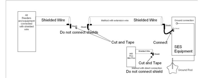
As the above drawing shows, grounding the card reader correctly is very important. Since the ground lug for the CAT is near the top of the unit, take care to avoid shorting the card reader cable shield to components on the mother board.
