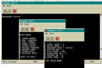
The Communications Setup menu comes with factory defaults that should be sufficient for most installations. These default values are shown on Pg. 51 and 52. Some functions are used with options that may not be present on your CAT. For example, selection 2 RS-232 Baud is not valid unless you purchase the optional serial printer interface (OPTKPRT). To get the right menu, press "4" from the main menu.
